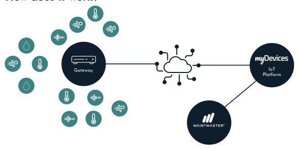
Sensors installed at your location periodically send data to the local IoT Gateway. The data is then sent encrypted over the internet to the myDevices IoT Platform. If the data triggers alerts, notifications are sent by email and/or SMS to the configured recipients. An integration with MaintMaster creates a maintenance job and refreshes the sensor site object in MaintMaster.
